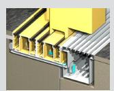
Can accept sliding door panels in a variety of commercial applications. This fully recessed sill is completely flat and still keeps water out. Complies with AS1428.
